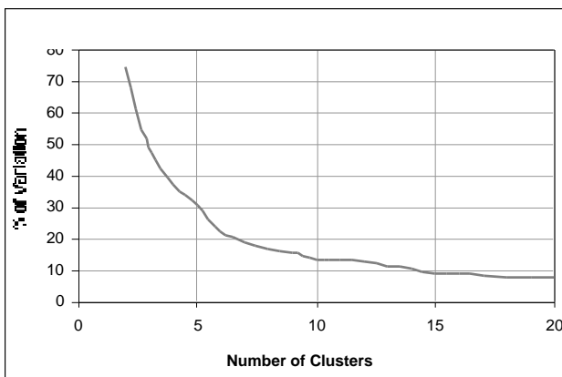
Figure 4. The percent of variation for various numbers of ISODATA-derived clusters used to determine the optimal number of final classes
