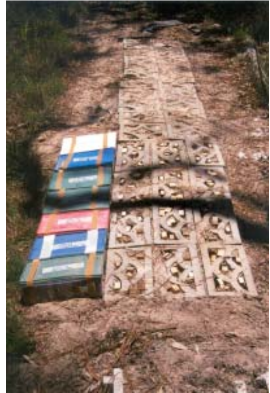
Figure 3. Concrete bricks were laid above the trench. Radiata pine feeder stakes were driven into gaps in the bricks to encourage movement of termites from the ground to the test specimens.
