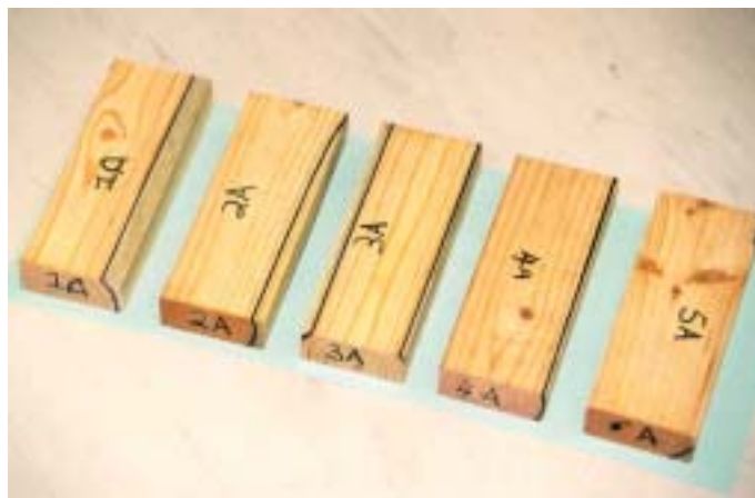
Figure 1. The boundaries of sapstain on maritime pine heartwood blocks marked on each block with a felt pen
