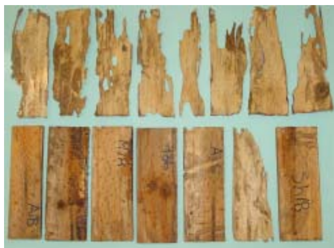
Figure 7. Damage caused by M. darwiniensis to feeder specimens (top row) and test specimens (bottom row): F 1 hybrid heartwood (4 samples), F 1 hybrid sapwood, slash pine sapwood and slash pine heartwood (left to right, respectively)
