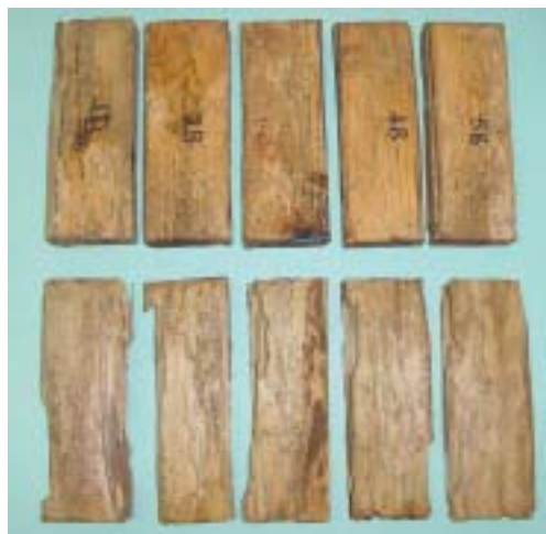
Figure 5. Damage caused by M. darwiniensis to maritime pine test specimens: heartwood (top row), sapwood (bottom row)
