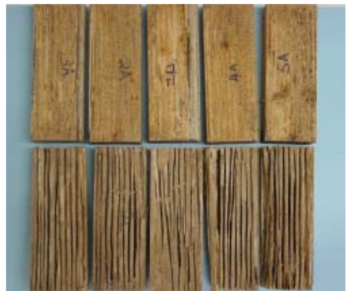
Figure 4. Damage caused by C. acinaciformis to maritime pine test specimens: heartwood (top row), sapwood (bottom row)
