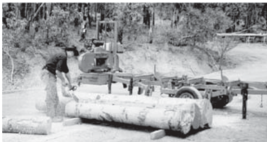
Figure 2. Paulownia logs being docked before sawing using a Wood-Mizer portable bandsaw mill
