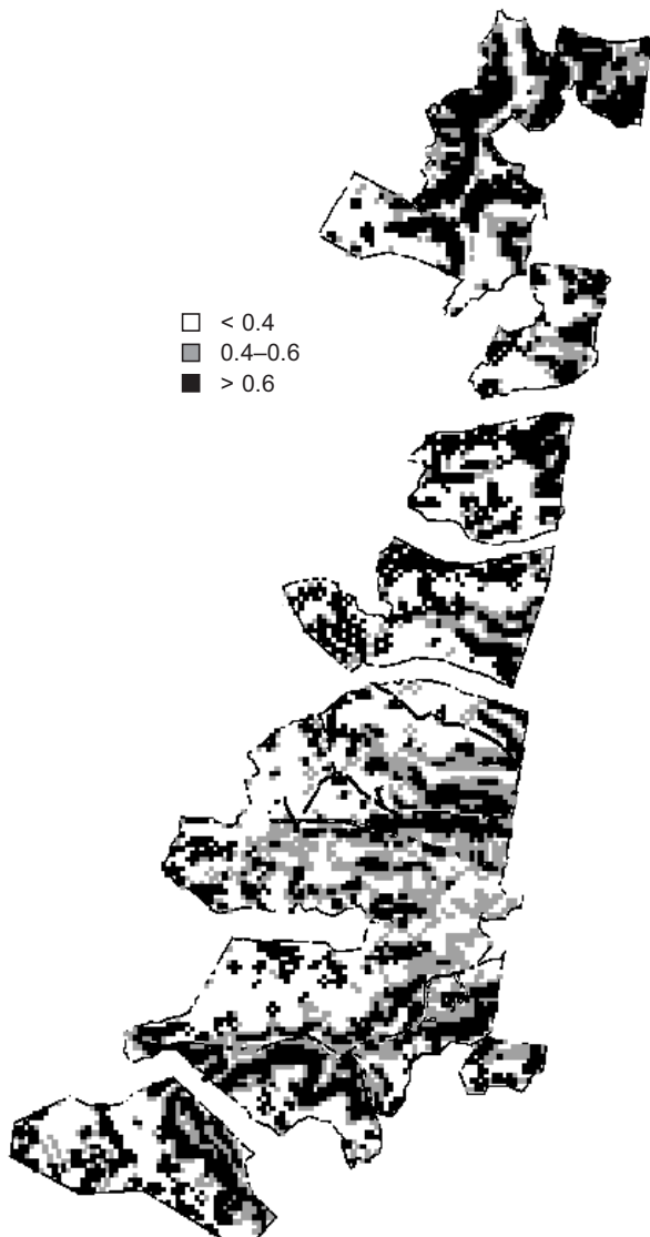
Figure 7. Map of vulnerability to landslides showing the MCE solution, based on the density of the drainage system (30%), slope (50%), geological units (10%) and structural features (10%)
