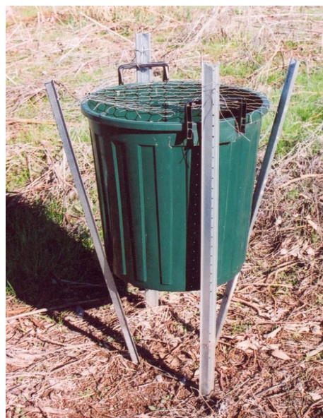
Figure 1. A modified garbage bin seed collector (127/25)
