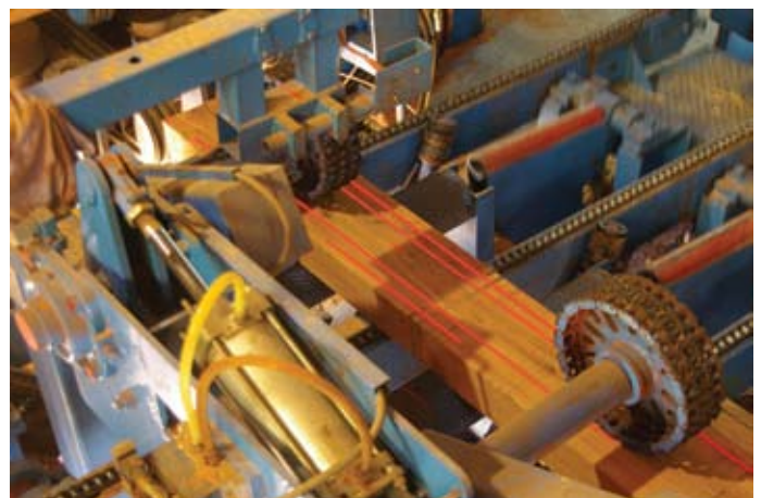
Figure 1. The system at Whittakers Timber Products processing 17-year-old pruned plantation-grown Eucalyptus saligna . Left: sawing on the twin band-saw; right: scanning of the central cant prior to sawing on the multi-saw.
