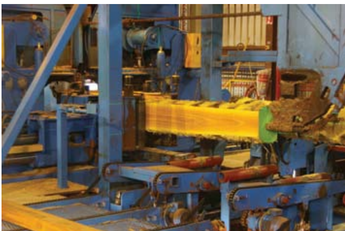
Figure 1. The system at Whittakers Timber Products processing 17-year-old pruned plantation-grown Eucalyptus saligna . Left: sawing on the twin band-saw; right: scanning of the central cant prior to sawing on the multi-saw.
