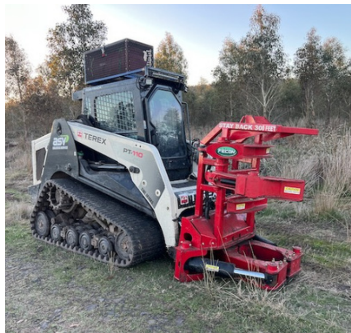
Image Two: Skid steer with harvesting shears and built in stump spray unit used for thinning demonstration.
