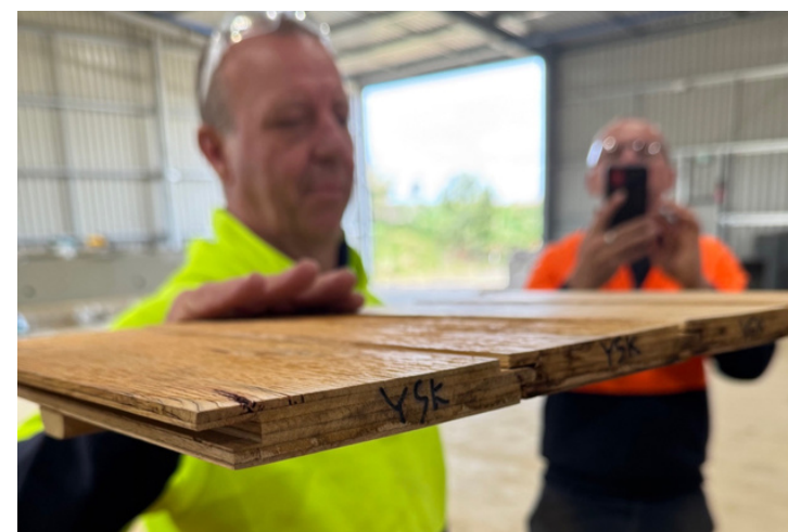
Image Four: Trial engineered shiplap using yellow stringybark veneer.
