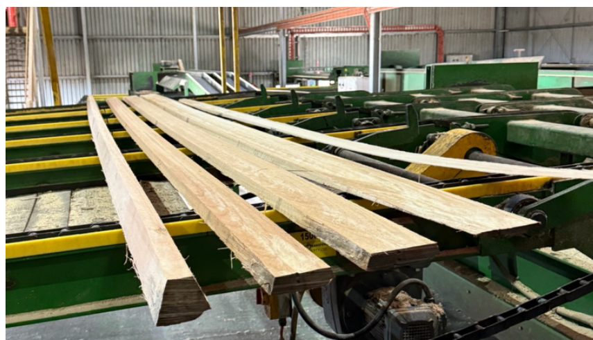
Image Five: Sawlog wedges back sawn into different width boards and screening products ready for moulding.
