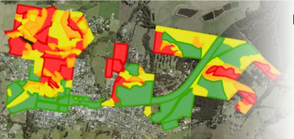
Damage mapped and classified from aerial / drone imagery
