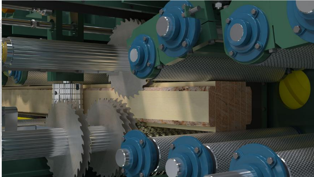
Internal view of a USNR Horizontal Shape Saw, capable of curve sawing and profiling a log cant in a single pass
