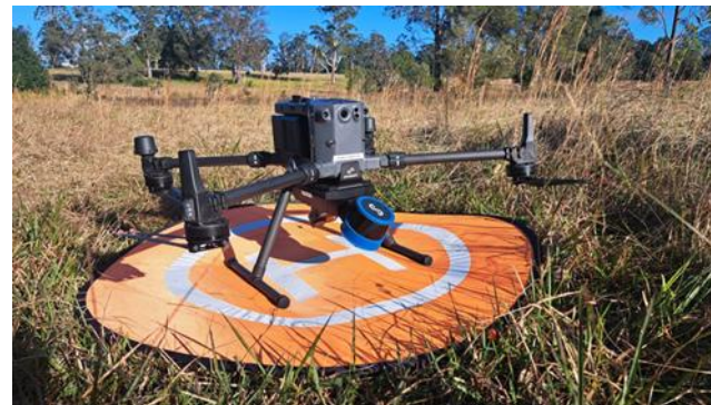
Drone (DJI Matrice 350) with the Hovermap ST-X onboard
