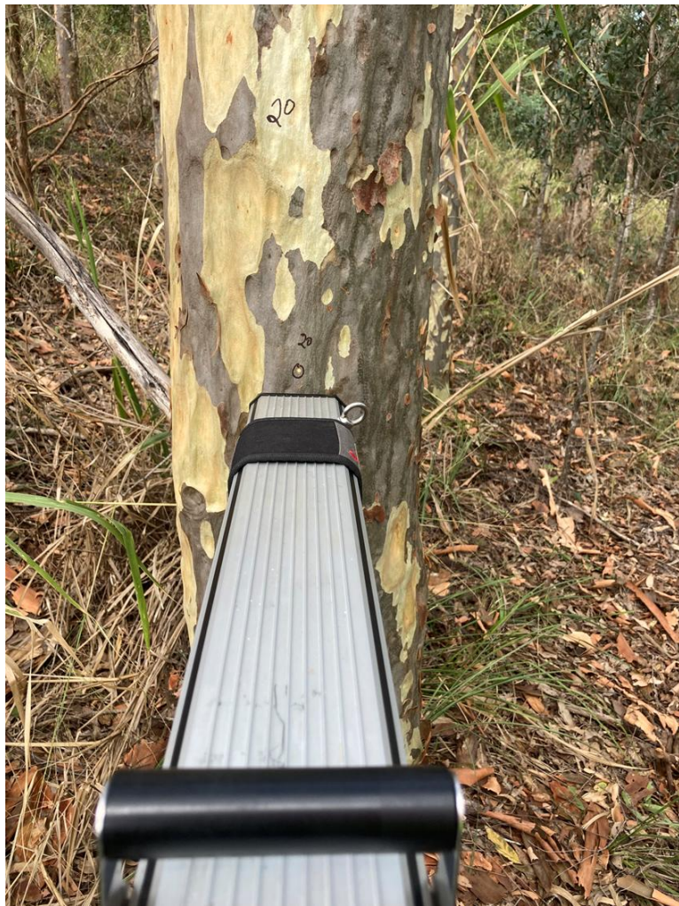
Drilling with IML Resi PD 500
